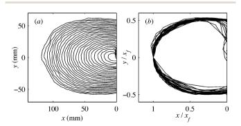
Fig. 5 Shape of the front plotted for different instances of time. Time difference between each line is 2.5 ms. Lines are drawn where the axial component of the velocity is half the pusher velocity (i.e.,  $u/u_p=\frac{1}{2}$ ). The origin of the coordinate system is defined as the instantaneous position of the pusher. (a): the evolution of the front during the experiment. (b): the same lines, normalized by the axial front position  $x_{\rm f}$ .
