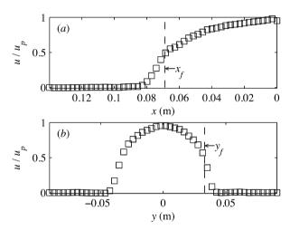
Fig. 3 Axial (a) and transverse (b) velocity profiles at t=17.5 ms along the lines indicated in Fig. 2b. The vertical dashed lines indicate the axial and transverse front position. The maximum slope du/dx of the axial velocity in (a) is approximately -14 s<sup>-1</sup>. At the transverse front position  $y_{\rm f}$ , the shear rate (slope of the velocity profile du/dy) is approximately 15 s<sup>-1</sup>.
